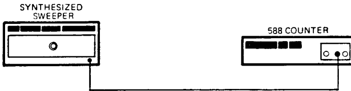
Figure 4-25. Band 2 Center Frequency Test Setup
